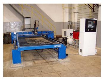
Destined for cutting of sheet metal on any contour. Are effectively used by diecutting of sheet metal in provision production of engineering plants and also for production of parts with complicated shape.
